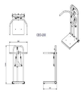
Side Bending Machine with hydraulic resistance mechanism
