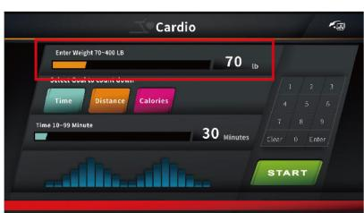
There are three goals which are Time, Distance and Calories. Choose one goal and set by adjusting the bar directly or clear number, then enter by numerical keys of the console.
