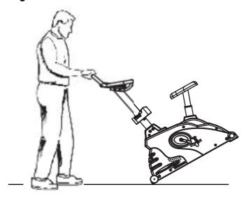
STEELFLEX upright cycle, firmly grasp the handlebars, carefully tip toward you and roll on the transport wheels.
